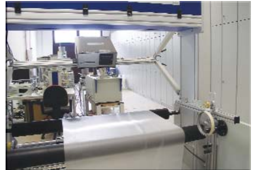
Speed measurement for quality control of films
