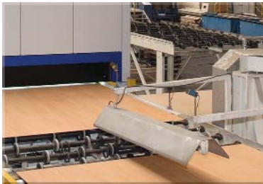
Length measurement in chipboard production
